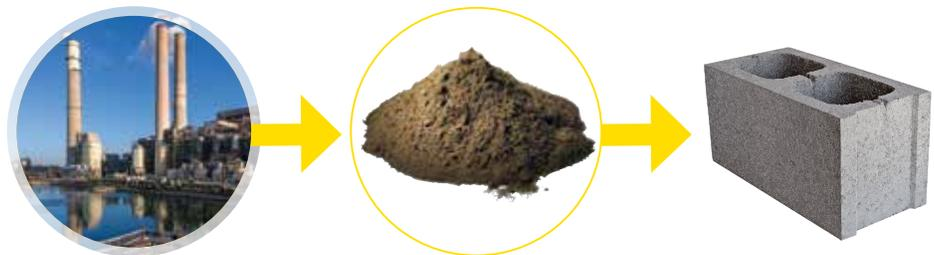
Fly ash is used to make cement and other concrete products.
